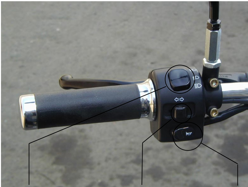
Low and High Beam Light Switch
