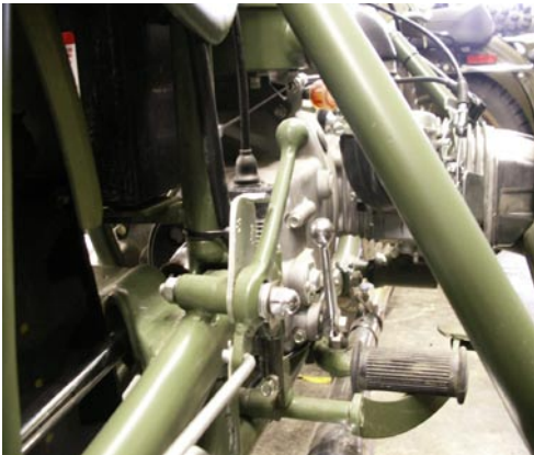
Sidecar Drive Disengaged
