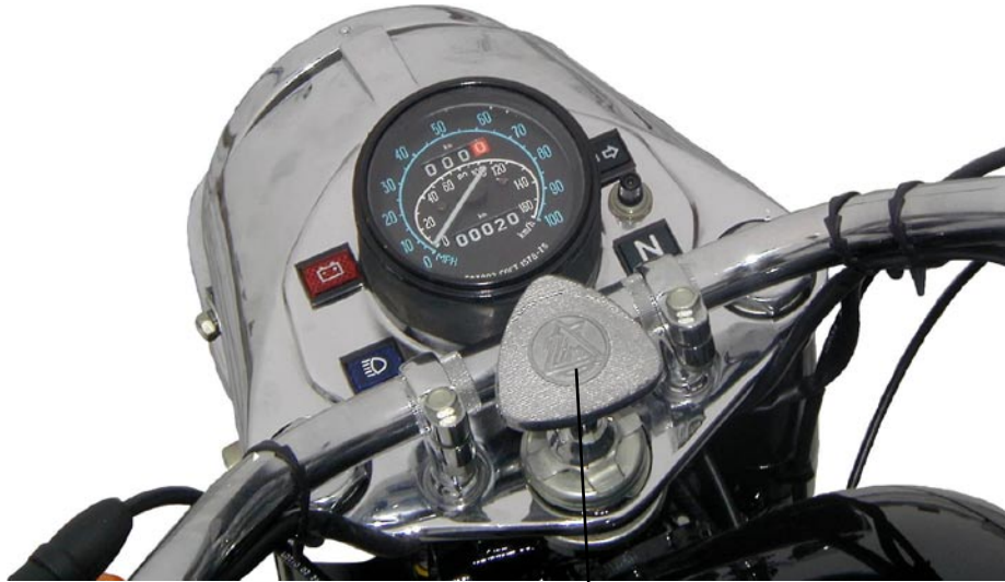
STEERING DAMPER ADJUSTMENT KNOB
