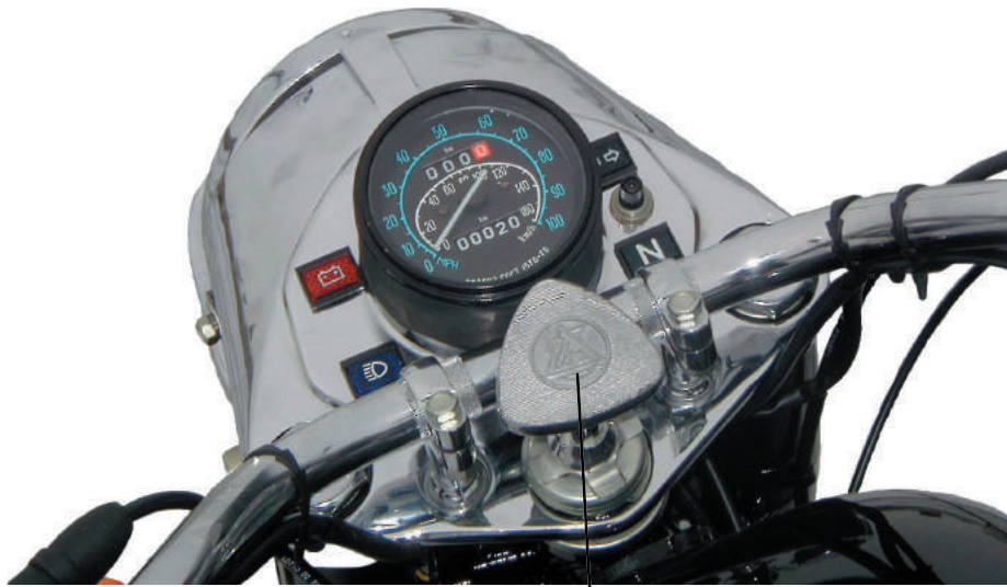
STEERING DAMPER ADJUSTMENT KNOB
